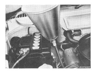
• Add additional oil through a fine-mesh funnel into guide tube of dipstick with the engine running.
